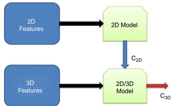
Figure 14. Cascade classifier flowchart.
