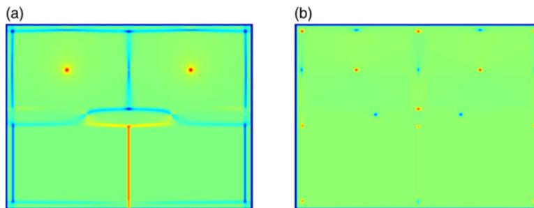
Figure 8. Graphical demonstration of correlation approach. (a) Cross-correlation result and (b) circular correlation result.
