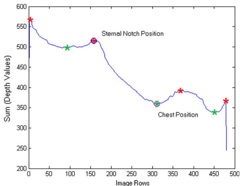
Figure 11. Sternal notch detection (red \* – local maximums; green \* – local minimums; blue circle – ST position; magenta circle – chest position).
